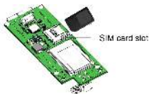
Figure 9: Inserting the card into the GSM modem
