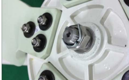
Insert the cotter into the shaft bore and separate the tails as shown.
