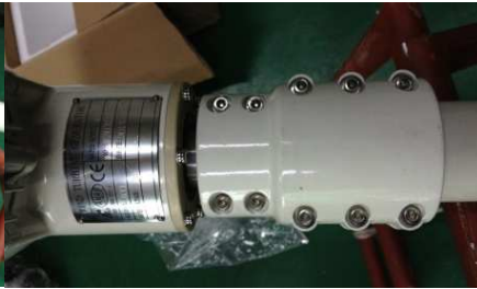
The pole is inserted into the lower part of the clamp.
