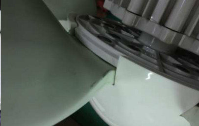
Place the hub with blades onto the rotor shaft. The place in sequence flat washer, spring washer and hex nut.
