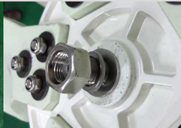
Place the hub with blades onto the rotor shaft. The place in sequence flat washer, spring washer and hex nut.
