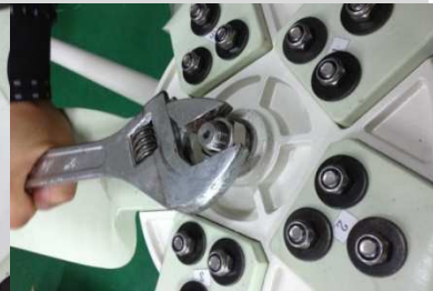
Fully tighten the nut with 154 Nm.
