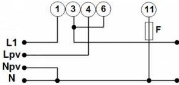
On the CCGX go to the grid meter in the Wired AC sensor settings. Make sure 'Phase type' is set to 'Single phase' and 'PV inverter on phase 2' is enabled.
