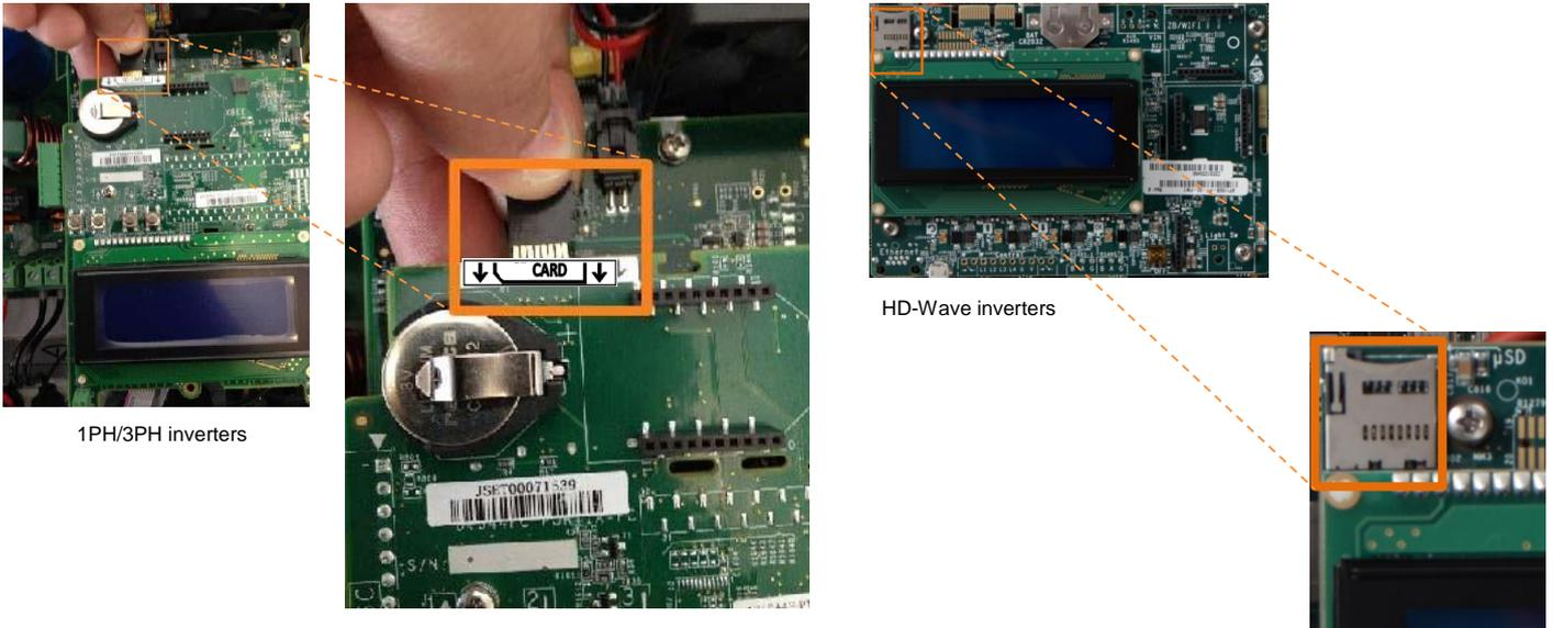
**Figure 2: Inserting the card**
