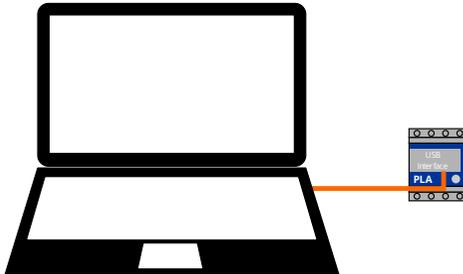
The laptop is connected directly to the interface via a USB cable.
