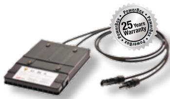
The SolarEdge power optimizer is integrated into each module, replacing the traditional junction box, or connected to it externally. The power optimizer optimizes energy output by performing MPPT for each module, and enables monitoring of each individual module. Further, each string's power optimizers automatically maintain a fixed string voltage, giving installers greater flexibility to design optimal PV systems.
