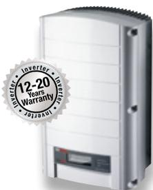
The SolarEdge inverter is a highly reliable inverter. Because MPPT and voltage management are handled separately for each module, the inverter is only responsible for DC to AC inversion. Consequently, it is a simpler, more reliable device. The fixed string voltage ensures operation at the highest efficiency at all times, independent of string length and temperature.
