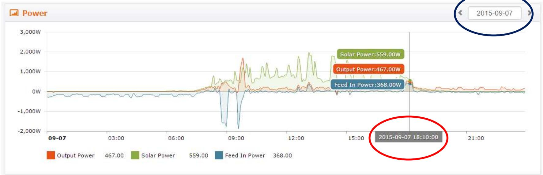
This is the main graph you will use, as you can see there are three main entities; **Solar Power**, **Output Power** and **Feed In Power**. All are measured in watts (W). The grey line represents what time of day you are looking at, as you can see in the image above we are looking at what is happening at **18:10:00** or **6.10pm** (circled in red) on the **07/09/15** (circled in blue). You can select a date by simply clicking the arrows either side of the date to choose another date.
