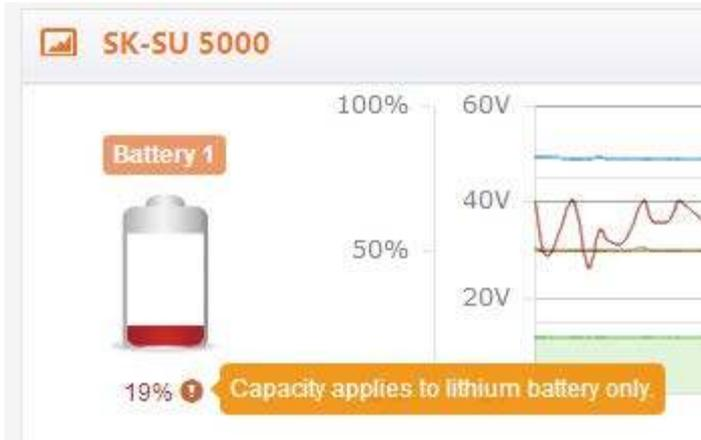
As you can see there is a small exclamation mark below the battery picture, when you move your mouse on the mark it will pop-out a reminder to tell you that Capacity only applies to Lithium batteries so if you do not have lithium batteries you will be limited to what you can see.
