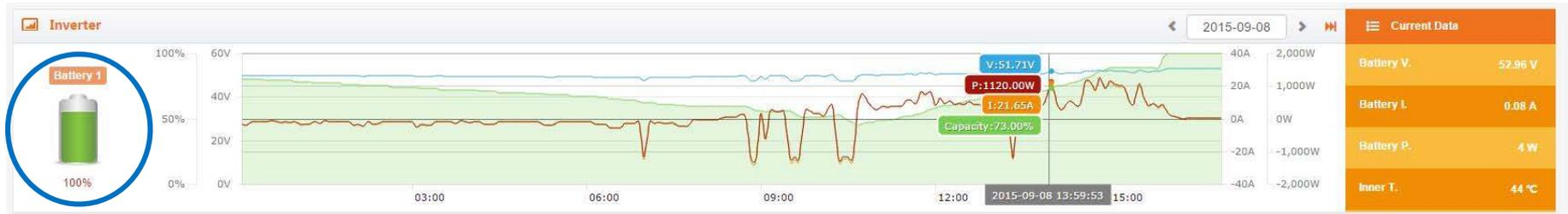
The battery image on the left (please note the 'Battery 1' is all of your batteries combined) gives you a clear indication of the amount of charge inside your battery, as you can see on this image (circled in blue), the battery is at 100%. \*Please note that the battery image is a real time reading so it will not correspond with the part of the graph I have highlighted.
