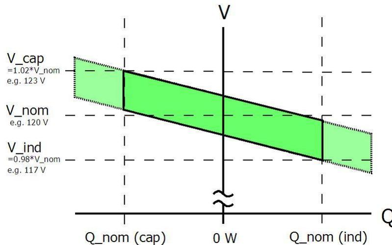
**Figure 4.2:** Generator behavior: voltage
