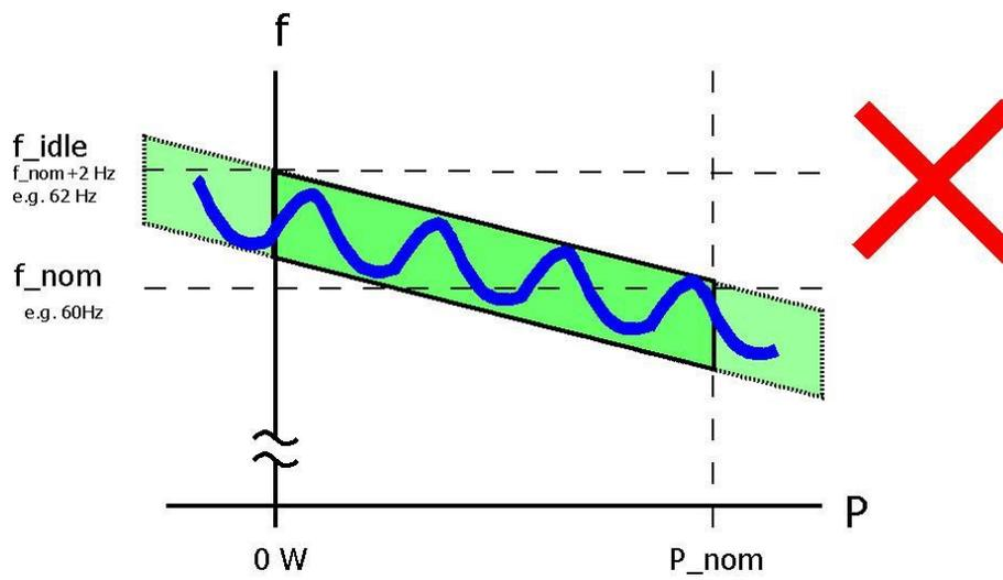
**Figure 8.4:** Generator behavior: discontinuous frequency - not suitable
