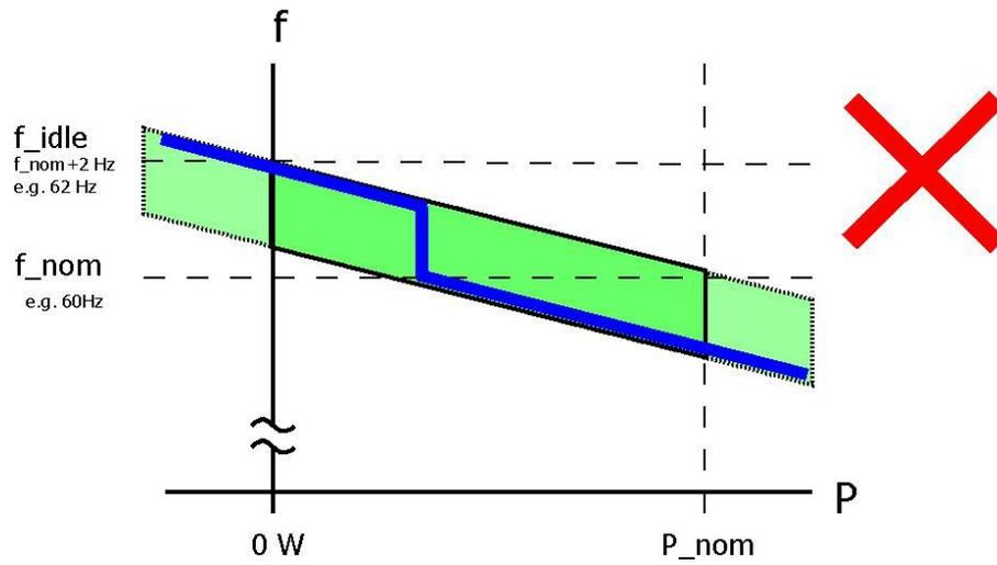
**Figure 8.3:** Generator behavior: frequency - discontinuous - not suitable
