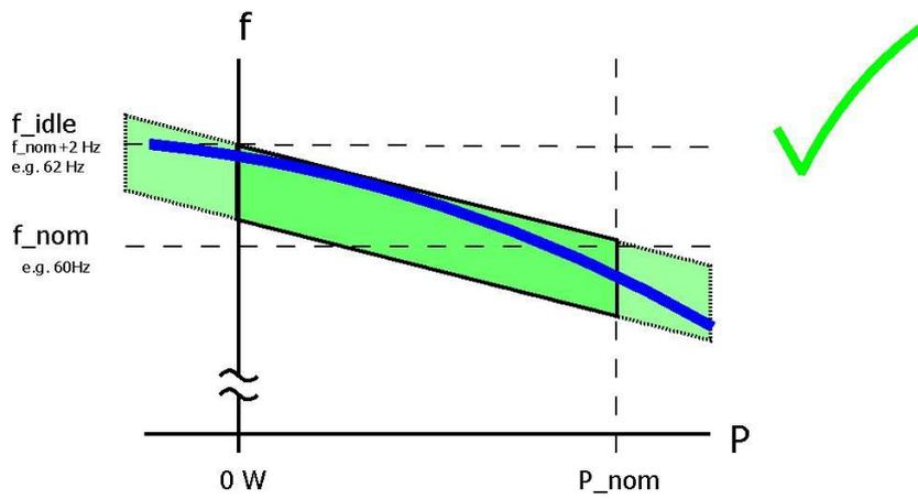
**Figure 8.2:** Generator behavior: frequency - continuous - suitable
