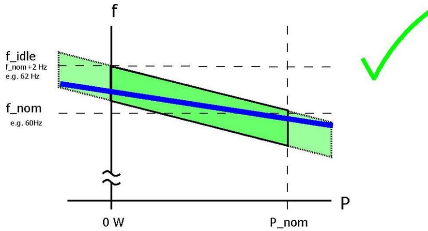
**Figure 8.1:** Generator behavior: frequency - linear - suitable
