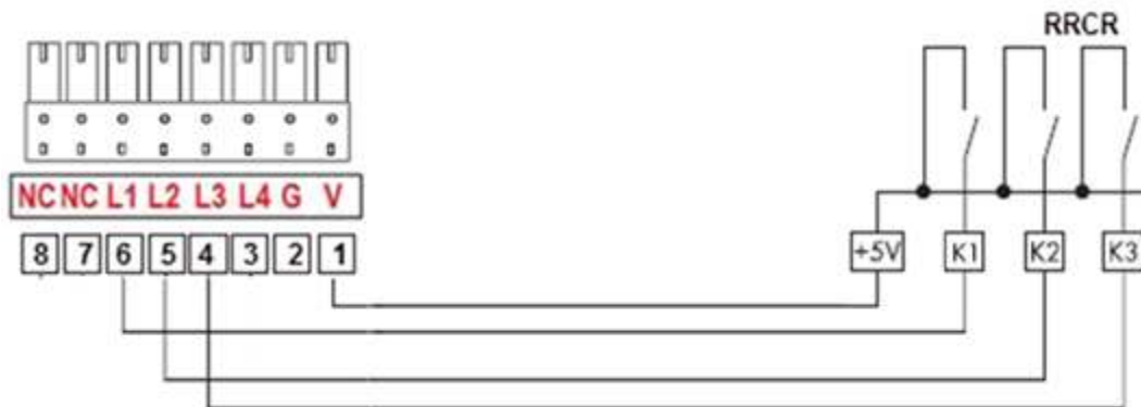
Figure 5 – Inverter – Three-Relay RRCR Connection
