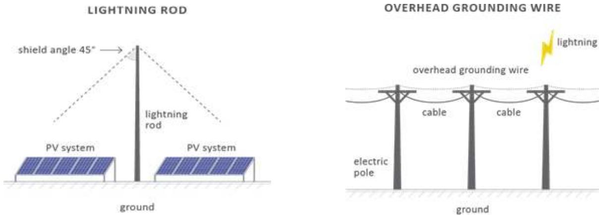
One effect of a direct lightning strike is increased ground potential – when the lightning strikes a building or a lightning rod, high current flows to the ground and the ground potential rises. This creates a potential difference between ground and external conductors, leading to surge behavior.
