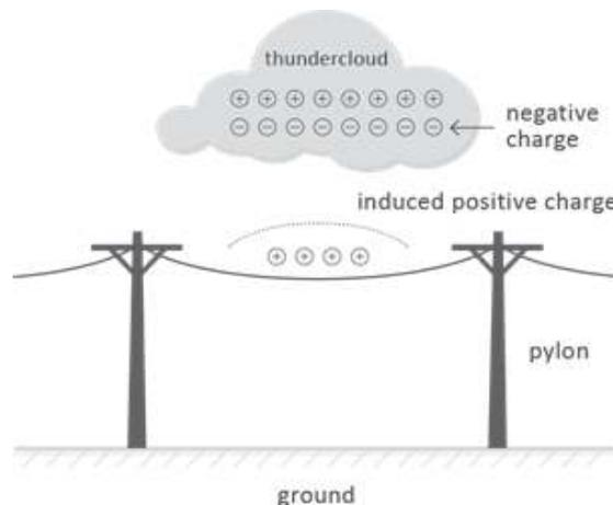
During discharge of the thundercloud (lightning), the positive charge accumulated in the cable is released, resulting in a surge in the cable in both directions.
