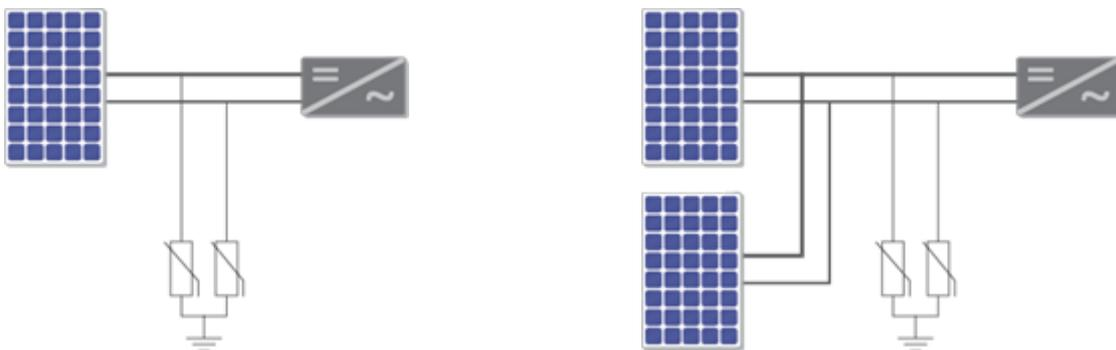
For inverters with an integrated fuse box, internal fuses should be bypassed in order to connect an SPD, and external string fuses should be connected.
