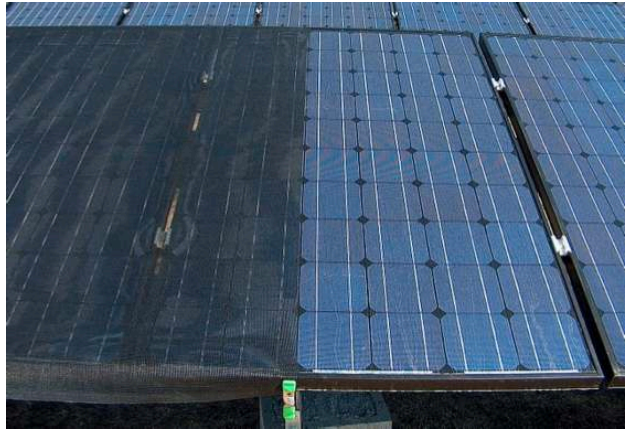
Figure 3: Semi-transparent mesh applied to solar modules to simulate shade.
