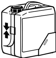
2. Fasten the belt on the fuel cartridge holder. Only connect EFOY fuel cartridges to the EFOY COMFORT fuel cell if they are secured with a fuel cartridge holder.
